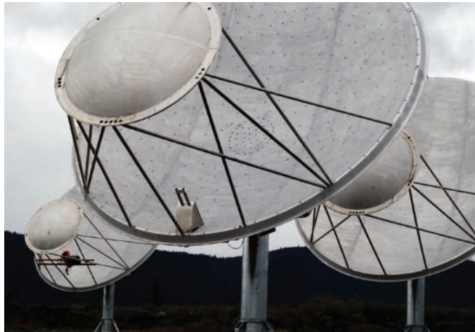
Listening for E.T. The SETI Institute is deploying an array of antennas and tying them into a giant "virtual telescope."
