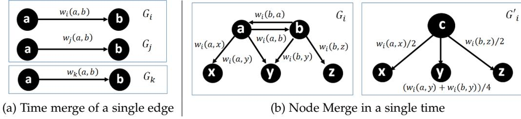
Fig. 2: (a) Example of merge operation on a single edge  $(a, b)$  when time-pair  $\{i, j\}$  is merged to form super-time  $k$ . (b) Example of node-pair  $\{a, b\}$  being merged in a single time  $i$  to form super-node  $c$ .
