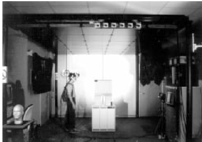
Figure 2: The University of North Carolina at Chapel Hill optical tracking system. The ceiling above the user is instrumented with a dense grid of LEDs. The system computes the users head position based on the set of LEDs visible to each of the cameras mounted on his head. (Courtesy of Ronald Azuma, University of North Carolina at Chapel Hill)
