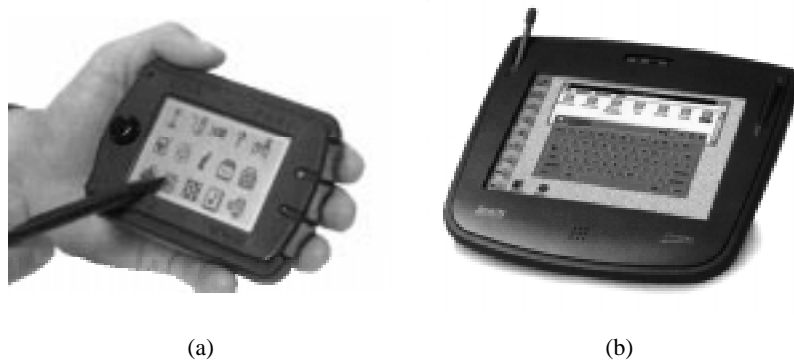
Figure 5: (a) The PARCTab is an example of a display used in a ubiquitous computing environment. It has a low resolution display, pen interface, three buttons and an infrared link for wireless communication. (Courtesy of Xerox PARC.) (b) The Zenith CruisePad is an example of a hand-held pad sized display. (Courtesy of Zenith Data Systems Corporation.)
