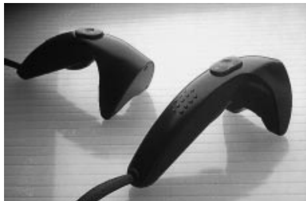
Figure 7: The Cricket, a 3D interaction device used in virtual environments. The flat front face of the left Cricket has three microphones for use with a 6DOF ultrasonic tracking system. The array of small circular bumps seen on the handle of the right Cricket provides haptic feedback. (Courtesy of Digital Image Design)
