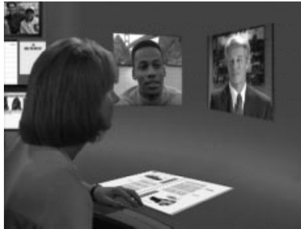
Figure 10: By rotating the images of the two remote participants in a video conference, the three participants could all see each other in the same relative positions. (Courtesy of Bruce Tognazzini, SunSoft)
