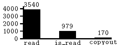
Figure 3: Overhead Reduction: 1 Byte HP-UX read versus is_read costs in CPU cycles
