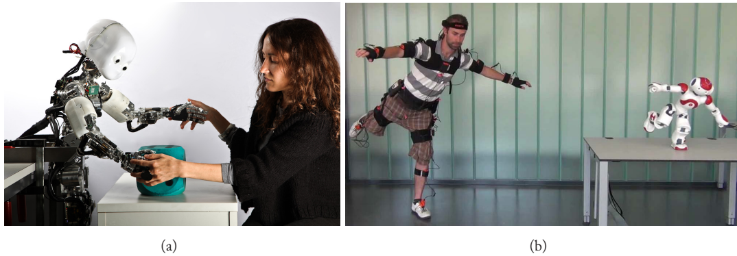
Figure 3.3: (a) Kinesthetic teaching with the iCub robot [13]. (b) User controlling the full-body motions of an Aldebaran Nao robot using the Xsens MVN inertial motion capture suit [141].
