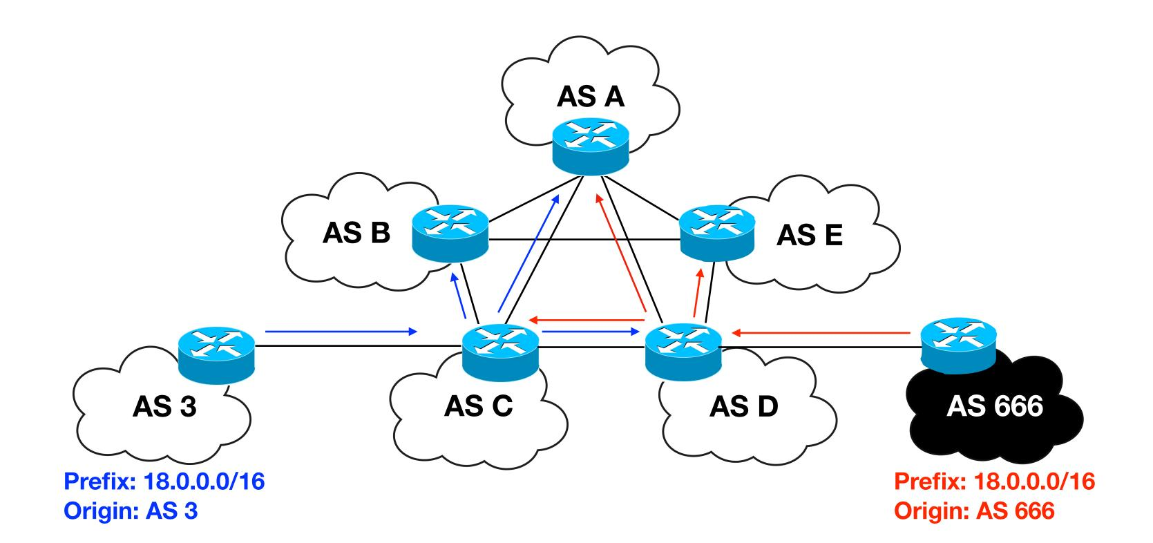
BGP lacks a mechanism for route validation.
