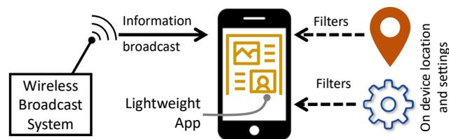
Figure 1: A light-weight app resides on the mobile phone. Information is fed from the wireless broadcast system and filtered on the mobile phone, based on location.
