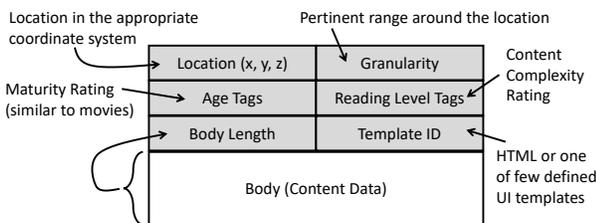
**Figure 2: An application level protocol to enable unidirectional broadcast information flow that contains sufficient information for rendering content on the mobile application.**
