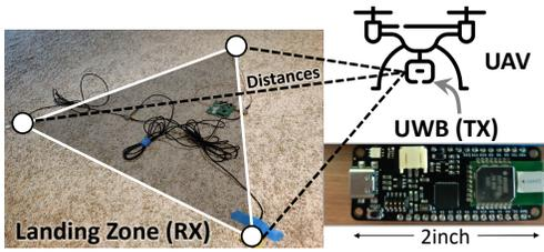
Figure 4: Homecoming test LZ ranging with UAV
