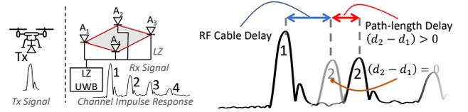
Figure 3: (a) UAV’s transmission arrives as multiple replicas at the LZ through each antenna. (b) Received signal copies capture the RF cable + path-length delay.
