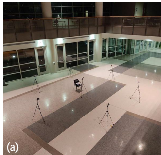
Fig. 2. Example implementation of PnPLoc : (a) UWB anchors mounted on tripods deployed in a building atrium; (b) UWB device used in demonstration; (c) User device with UWB tag attached to a mobile phone.
