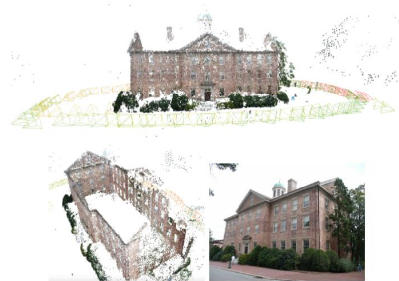
Figure 1. A sparse reconstruction of the UNC South Building using GTSfM with a deep LoFTR-based [64] front-end, with an example image input. Multi-view stereo is not used.
