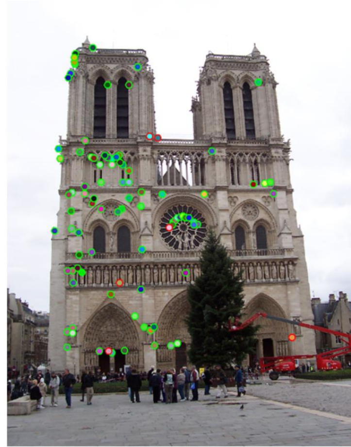
The top 100 most confident local feature matches from a baseline implementation of project 2. In this case, 93 were correct (highlighted in green) and 7 were incorrect (highlighted in red).
