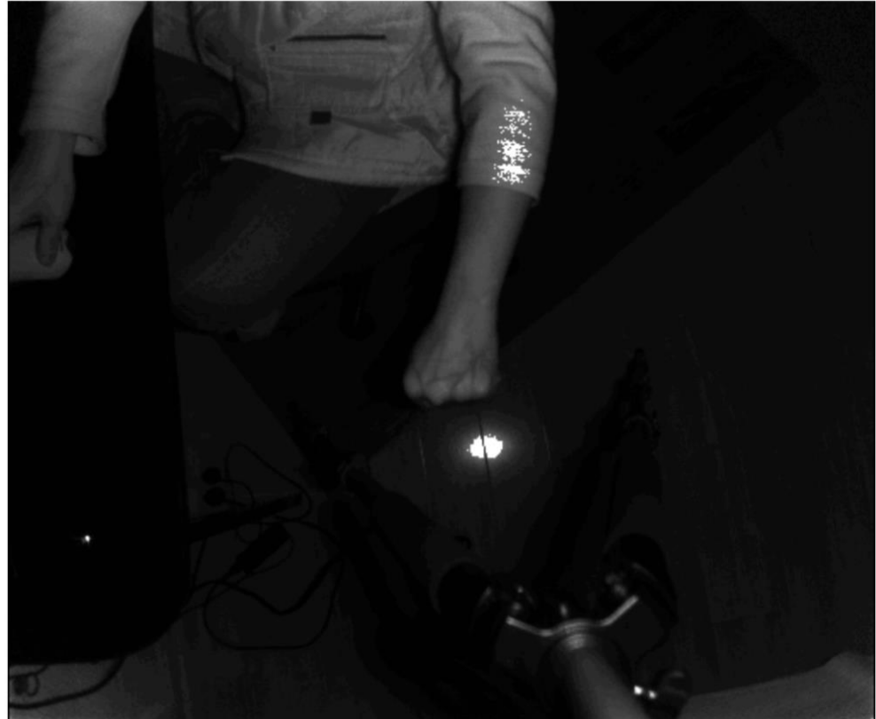
Infrared images of Kinect V1 structured light pattern and Kinect V2 time of flight pattern. Credit "Lightweight Algorithms for Depth Sensor Equipped Embedded Devices" by Henry Zhong
