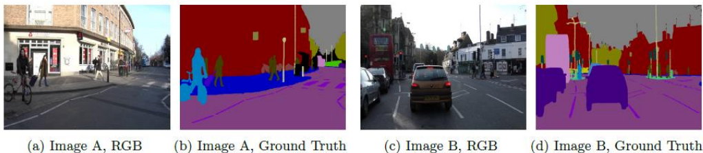
Figure 2: Example scenes from the Camvid dataset. The RGB image is shown on the left, and the corresponding ground truth “label map” is shown on the right.
