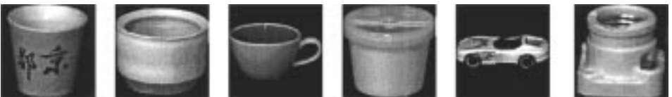
FIG. 12. Gross errors in the orientation determination are mainly caused by rotation-symmetric objects.
