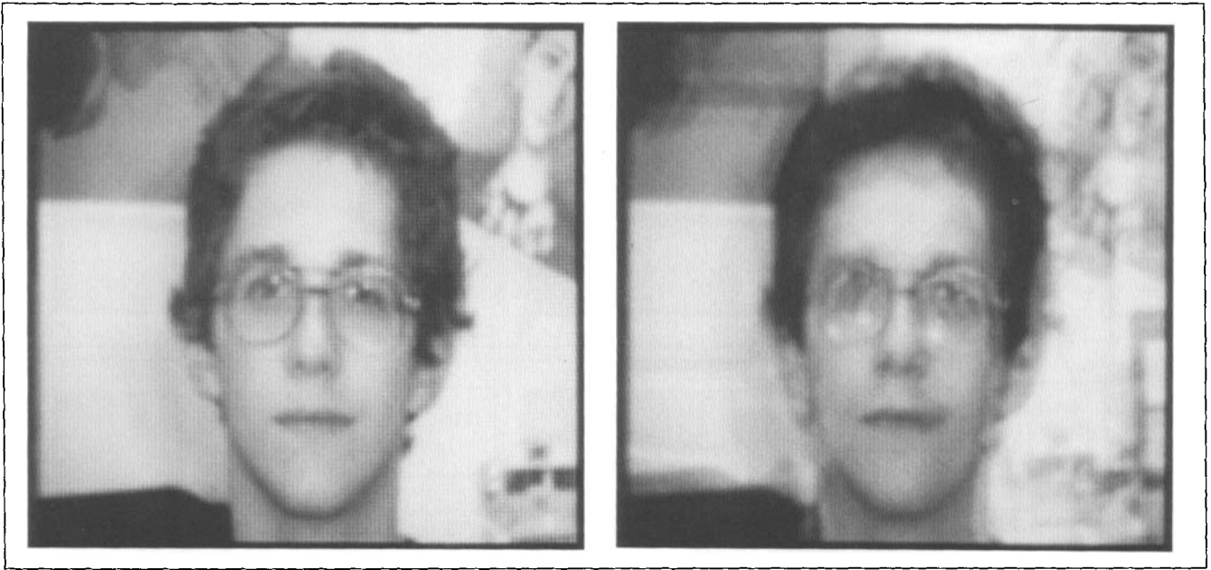
Figure 3. An original face image and its projection onto the face space defined by the eigenfaces of Figure 2.
