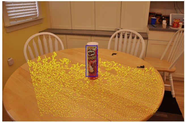
Fig. 3. Point cloud data is projected into the camera image. Horizontal planes are extracted (yellow points) and objects are clustered points which appear above the plane (green points). The region of interest is selected based upon the projection of object points into the image (blue rectangle)
