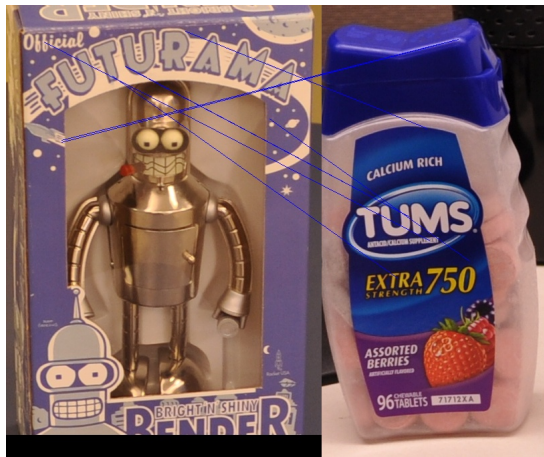
Fig. 5. An object which does not match with class "Sundries". The model image appears on the right, and the candidate object image appears on the left. Blue lines indicate matches which are inliers to the homography filter. There are too few inlier matches, so the recognition algorithm rejects this as a match.
