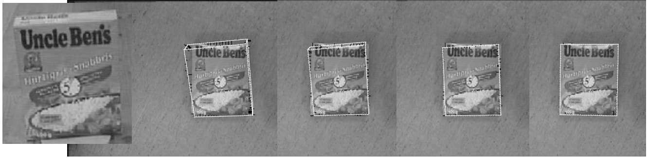
Fig. 12. Training image used to estimate the initial pose (far left) followed by the intermediate images of the fitting step.
