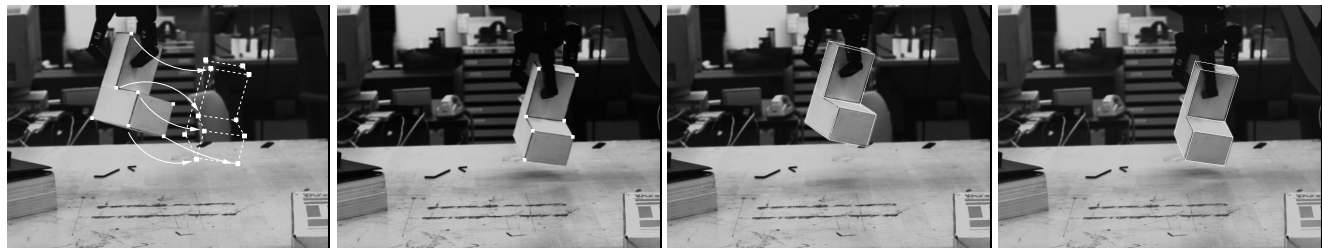
Fig. 15. Start pose, destination pose and two intermediate poses in an image-based visual servo approach.
