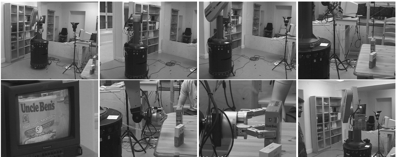
Fig. 16. An experiment where the robot moves up to the table, recognizes the rice box, approaches it, picks it up and hands it over to the user.
