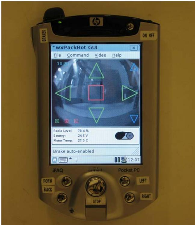
Fig. 2 The PDA running the graphical user-interface developed for the project.
