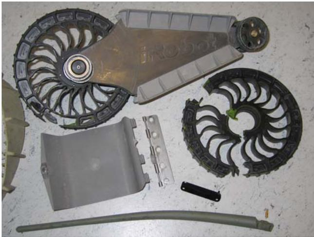
Fig. 7 Although the Packbot is fairly sturdy we experienced that it has its limits just above the drop-limit of two meters the manufacturer guarantees. On the top a broken Flipper arm, in the center holders and lid for one of the batteries and in the bottom an antenna that came off its connector and holder due to flip overs.
