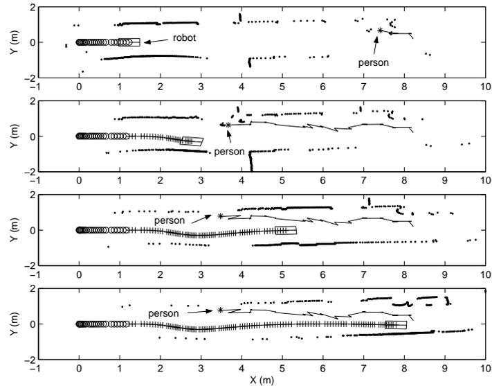
**Fig. 5.** The person walks along the corridor. The circles and the plus symbols represent the robot trajectory in ND and in PP mode, respectively. The person trajectory is shown as a continuous line and the star represents the person’s current position. The current obstacle points on the local map are shown as dots. The robot steers to the right to pass the person and then resumes its course.
