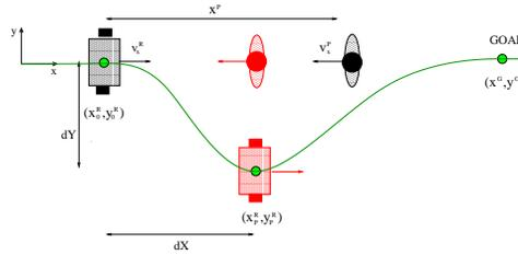
**Fig. 4.** Desired trajectory for the passage maneuver. The distance of the robot from the person is maximum when it is passing her/him (red).
