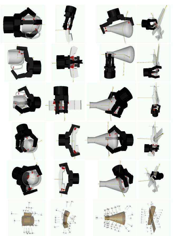
Figure 5: Planned grasps for a coffee mug, a phone handset, an Erlenmeyer flask, and a model airplane. The first image in each row shows the primitive model used for each object and the generated set of grasps to be tested. The other images show four of the best grasps found sorted in quality order.
