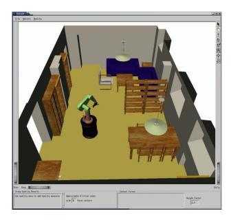
Figure 1: The GraspIt! system allows the importation of a robotic platform and model of the world in which it operates. In this case it is the manipulation platform and living room environment at the Center for Autonomous Systems. The furniture serves as obstacles in the grasp planning.
