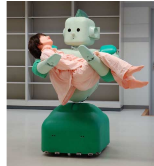
Fig. 1. RI-MAN is a platform for physical human–robot interaction research.
