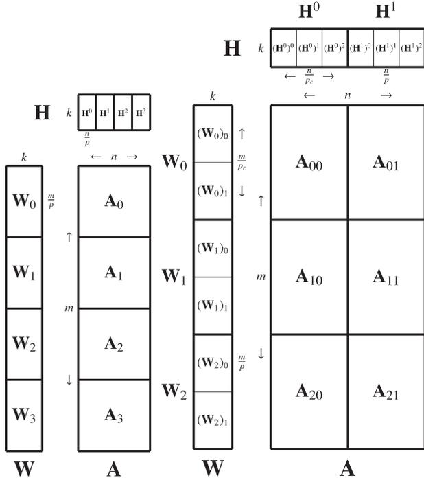
Fig. 2. Data distributions for MPI-FAUN. 1D Distribution on left with  $p = p_r = 4$  and  $p_c = 1$ . 2D Distribution on right with  $p_r = 3$  and  $p_c = 2$ . Note that for the 2D distribution,  $\mathbf{A}_{ij}$  is  $m/p_r \times m/p_c$ ,  $\mathbf{W}_i$  is  $m/p_r \times k$ ,  $(\mathbf{W}_i)_j$  is  $m/p \times k$ ,  $\mathbf{H}_j$  is  $k \times n/p_c$ , and  $(\mathbf{H}^i)^j$  is  $k \times n/p$ .
