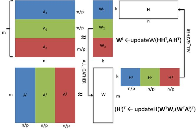
Fig. 1. Naive-Parallel-AUNMF. Both rows and columns of  $A$  are 1D distributed. The algorithm works by (all-)gathering the entire fixed factor matrix to each processor and then performing the Local Update Computations to update the variable factor matrix.
