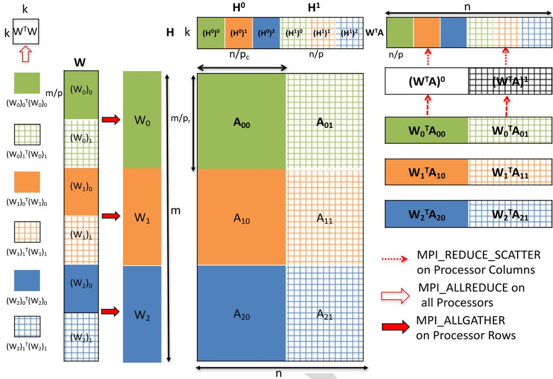
Fig. 3. Parallel matrix multiplications within MPI-FAUN for finding  $H$  given  $W$ , with  $p_r = 3$  and  $p_c = 2$ . The computation of  $W^T W$  appears on the far left; the rest of the figure depicts computation of  $W^T A$ .
