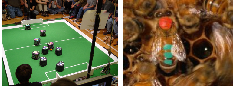
Figure 1: Multi-target tracking in robot soccer and social animal research. Left: In the RoboCup small size league robots are tracked using an overhead camera (image courtesy Carnegie Mellon). Right: A marked honey bee is tracked in an observation hive.
