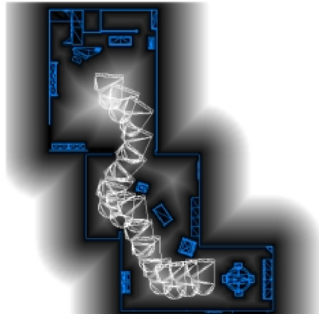
Plate 2: We create a potential field from the Voronoi diagram of the house floorplan to plan the motion of a piano through a complex static scene in real-time. Left: The piano motion sequence. Right: Motion sequence overlaying the floorplan distance function. The video demonstrates navigation through a dynamic scene in real-time.
