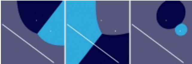
Figure 11: Standard nearest-site Voronoi regions (left). Farthest regions for the same sites (middle). Weighted regions (right). Weights: line, 2; dark point, 1; light point, 0.5.
