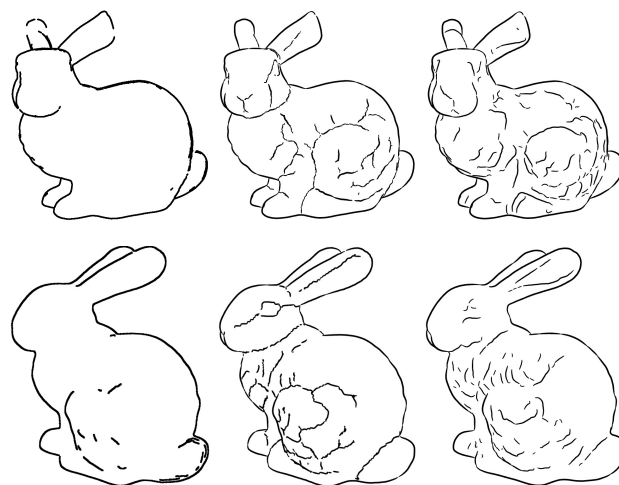
Figure 13: Comparison of several visual effects (two views of each): Left: edge detection applied to the depth map to extract depth discontinuities. Center: contours with valley lines computed as local maxima of curvature. Right: contours with suggestive contours computed using the object-space algorithm.
