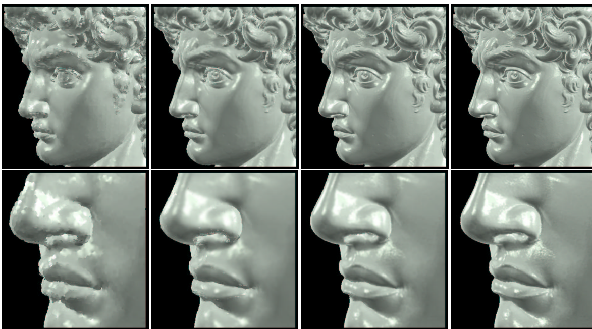
Figure 13: Progressive transmission of the David head model. From left to right we show snapshots with 5, 15, 50, and 100 percent of the data received. Reconstruction is done by breadth-first traversal. The bottom row shows close-up views of the top row.
