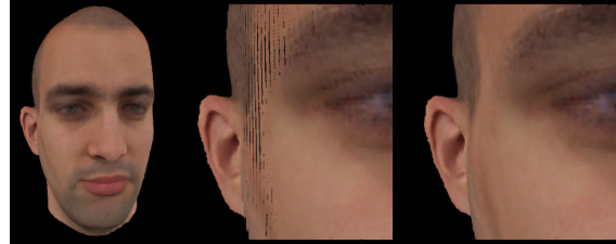
Figure 9: In flat areas viewed from a grazing angle gaps can appear because splatting fills holes only in tangential direction (center). Offset attributes remove these artifacts (right). In this example we use 2 bit precision for the offsets. Notice that we chose a very coarse PBR with only 198 K points (8 octree levels) to make the effect clearly visible in the center image. Normally this effect is much more subtle, affecting only a view scattered pixels.
