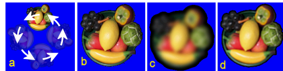
Figure 5: Test of dissipation and diffusion with image advection problem on a rotating vector field ( 800 \times 800 grid, CFL = 6.29 ). (b) is the top center portion of the original image (a). (c) is obtained by rotating it 360 degree using the first order semi-Lagrangian scheme, where one can see large amount of dissipation, diffusion, shrinkage of image and position error. These are significantly improved in (d) where BFECC is used. The blue background region is in fact in black color but it is rendered as blue to illustrate the region where the color is not diffused into.
