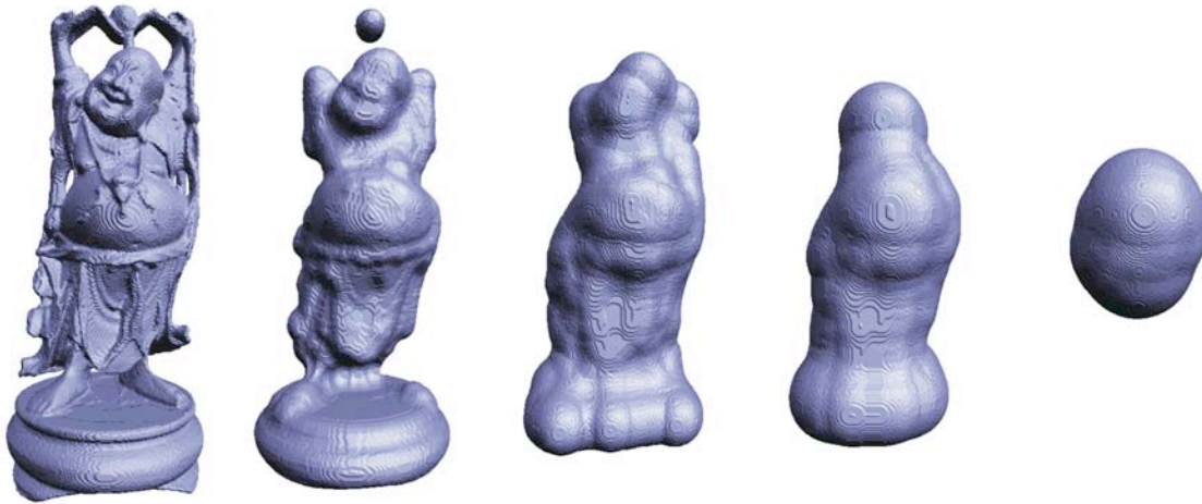
Figure 10: (Left to right) The original shape S and the results of applying Mason with radii of 16, 32, 48, and 64 voxels.
