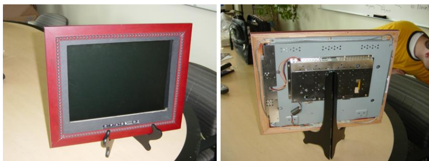
LCD – bezel + picture frame
