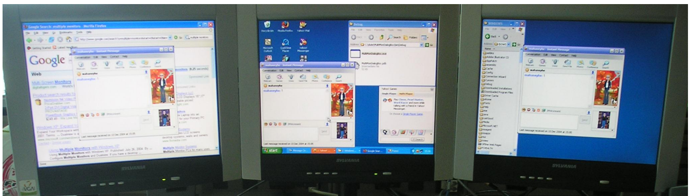
Figure 1. mudibo facilitates the appearance of a new incoming instant message on all three monitors of a multiple-monitor system. Monitor resolution has been decreased for visual effect. Typically, IM windows are much smaller and thus easier to miss.
