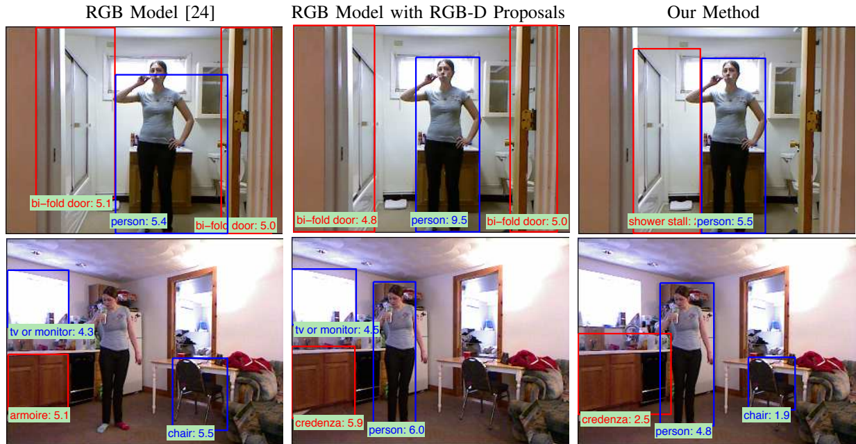
Fig. 6. We use our algorithm to transform the publicly available 7.6k class RGB detector [24] into an RGB-D detector. We show here detection results for all 7.6k categories on example RGB-D images taken from two scenes in the Cornell activity dataset [45]. We present top detections from the original RGB CNN with RGB selective search region proposals ( left ), detections when using RGB-D MCG proposals ( middle ), and detections after our proposed adaptation ( right ). Blue boxes are detections of the 200 ILSVRC categories, while the red boxes are detections of the 7.4k categories corresponding to leaf nodes in the ImageNet database. Our algorithm not only provides better localization, but even enables extra categories to be detected.
