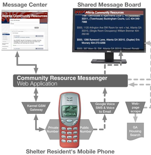
**Figure 6: Final CRM system architecture.**
