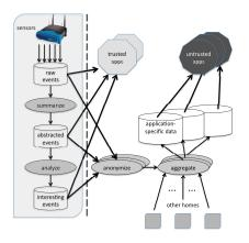
Figure 2: System architecture
