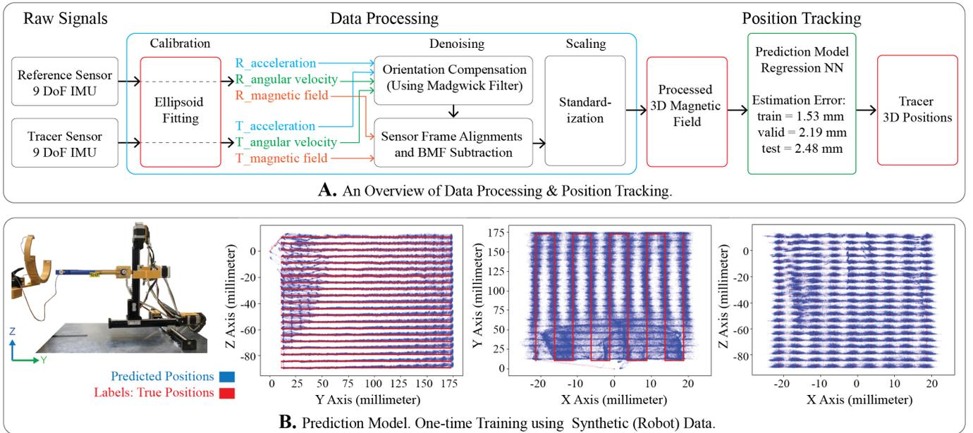
Figure 2. A. An overview of the data processing pipeline and position tracking algorithm. B. Using a 5DoF robot arm to collect synthetic data and train the position tracking model. Comparing predicted positions against true labels indicates 2.48 mm error (third quartile) in test data.
