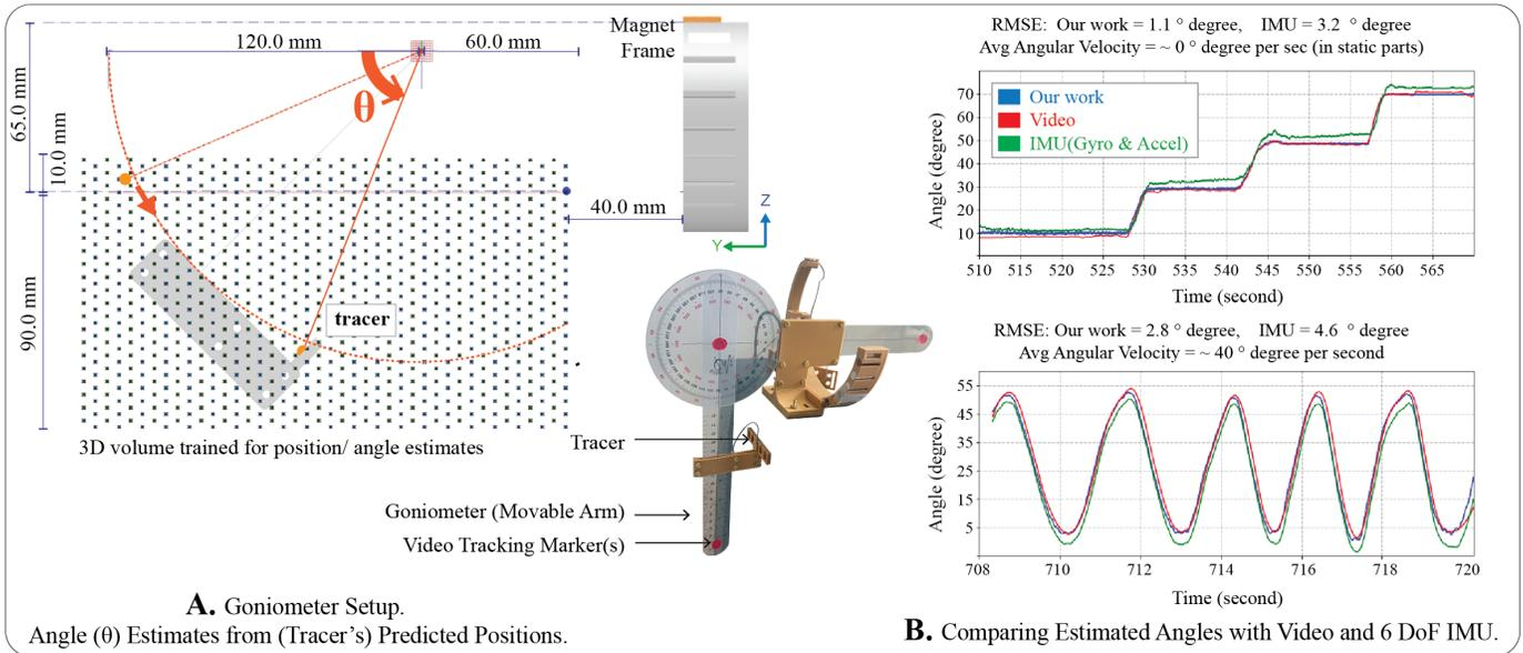
Figure 3. A. Goniometer setup shows the conversion of predicted (tracer's) positions into joint angles. B. Goniometer is equipped with the sensing hardware and tracer's static and dynamic motions are measured and compared against a commonly-used 6 DoF IMU and computer vision angle tracking method. Figure shows an illustrative example of angle estimates from two study sessions.
