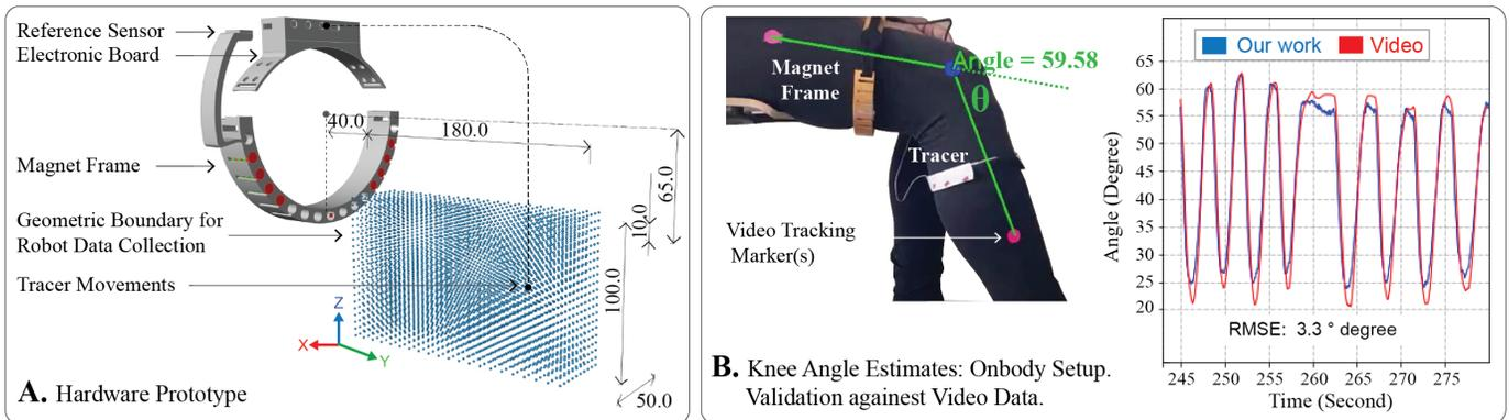
Figure 1. A. Our sensing prototype and the geometric volume in which the position tracking algorithm is trained. B. Knee angle estimates and their validation against a computer vision angle tracking method. Figure shows an illustrative example of angle estimates from one study session.
