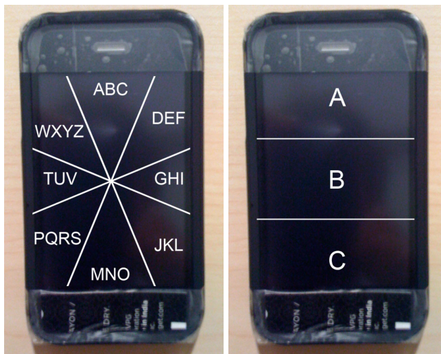
Fig. 2. No-Look Notes. The screen on the left is the main screen. The screen on the right is after the ‘ABC’ target is selected from the main screen. Visual representation was added to this figure for illustration.
