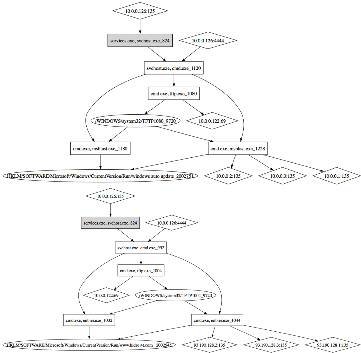
Figure 5.6: The information flow graph, rooted at svchost.exe, for the A and F variants of the Blaster worm on a Windows XP honeypot.
