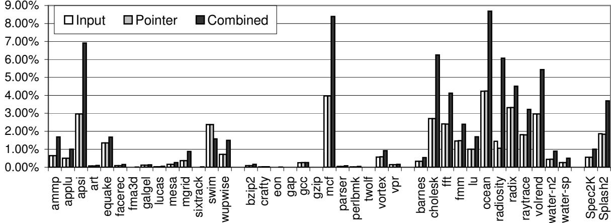
**Figure 5. Performance overhead of taint propagation with FlexiTaint.**
