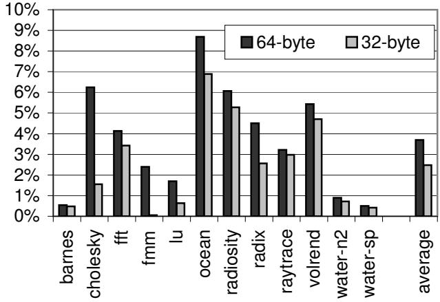
**Figure 8. Effect of TL1 line size in Splash-2.**
