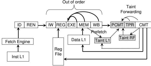
**Figure 2. Processor pipeline with FlexiTaint**
