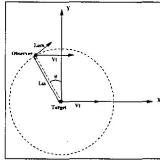
Fig. 3. Observer rotational motion around the target
