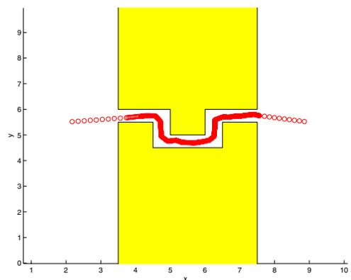
Fig. 3. Experimental setting: environment containing a narrow passage and a point robot moving through it.
