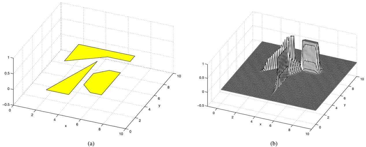
Fig. 1. Validation of the biasing scheme: experimental obstacle layout in (a) and the corresponding passage potential function in (b).
