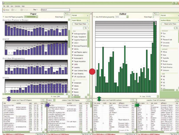
Figure 1 NetLens has two symmetric windows. The left is for Content (papers) and the right for Actors (authors). Each side is further divided into panels; overview at the top, filters on the right, and lists at the bottom. Here, the Content side has two lists to reflect papers and their citations or references, and the lists on the Actor side show authors and their co-authors, respectively. The paper overview panel shows the distribution of papers (in logarithmic scale) over time, grouped by topics. Users can see which topics have their number of papers increase or decrease over 22 years. On the right side, the overview of the authors shows the distribution of countries of origin in logarithmic scale.
