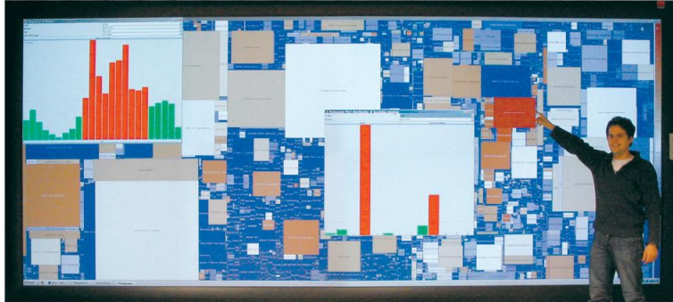
Fig. 5. Hierarchical Network Map displaying all 19,731 autonomous systems (one can still zoom in twice for details) on a large display wall (5.20m × 2.15m, 8.9 Megapixels, powered by eight projectors). The query interface on the top left shows the traffic distribution over time and specifies the selected data, in this case the traffic entering the gateway of the University of Konstanz on well-known ports (0-1023) on 29 November 2005 using "transferred bytes" as measure with logarithmic color mapping. One recognizes a heavy traffic load from AS 3320 (red) of "Deutsche Telekom" as well as to neighboring autonomous systems in Germany. A port histogram reveals high activity on the Web ports 80 and 443. For security and privacy reasons, the data was aggregated and sanitized.
