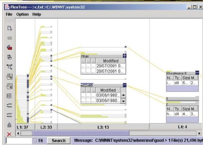
Figure 9 Zooming into multiple foci of interest within the context of the hierarchy. This demonstrates how the user can zoom into a tree and generate details on demand. The  $w32 \times 86$  node itself is shown in blue, rather than yellow as the other nodes, because all files in this folder were modified in 1980, which is much earlier than files in the other folders.
