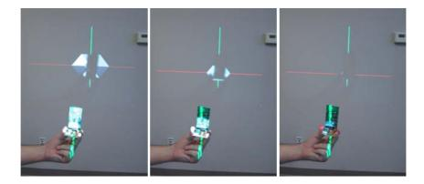
**Fig. 5.** Three frames from a video of the tracking pattern "zeroing-in" on a near-static sensor. The pattern size was artificially increased at the beginning of this sequence by covering the sensor for two seconds. For purposes of illustration our system is projecting red (horizontal) and green (vertical) lines which cross at the detected location of the sensor
