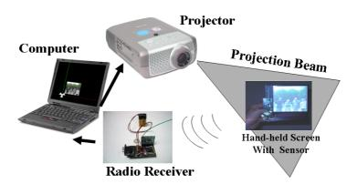
**Fig. 1.** System Diagram - While moving, a sensor on the hand-held screen detects location information from the projector and broadcasts it over the radio. A radio receiver returns this information to the computer, which adjusts the display accordingly to keep the projected image on the screen
