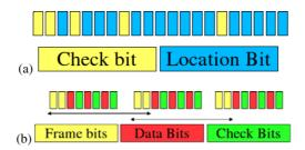
**Fig. 4.** (a) 21 bit location packet showing 5 check bits and 16 data bits, (b) A stream of three 8 bit tracking packets showing framing bits, data bits, and check bits. Arrows indicate the 10 bit pattern that is decoded, which includes framing bits at each end
