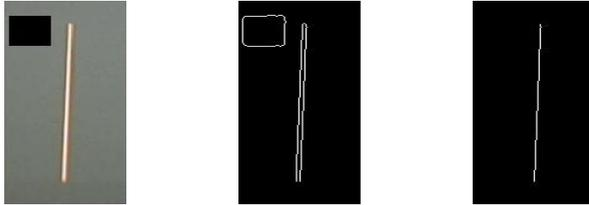
**Fig. 2.** Left: A line projected onto a wall and a black square representing an object in the environment. Middle: Results obtained applying Canny edge detection to the image on the left. Right: Result obtained applying the gradient based edge detection algorithm we developed.
