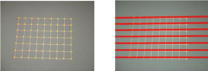
**Fig. 4.** Left: A projected grid. The yellow dots show points of intersecting lines. Right: Left image superimposed with epipolar lines.
