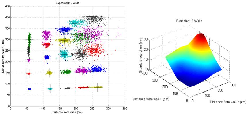
**Fig. 9.** Two wall experiment. Left: Each dot represents a single data sample. Dots of the same color belong to the same position data set and black crosshairs show mean values. Right: Up front view of interpolated standard deviation of the two wall readings.
