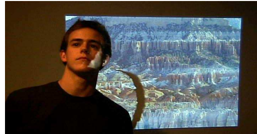
Figure 7. Active Virtual Rear Projection system with Blinding Light Suppression, with a moving user.
