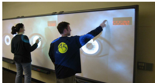
Figure 1: An interactive game using redundant illumination provided by GVU-PROCAMS. The redundant illumination prevents shadows from hampering the game-play.
