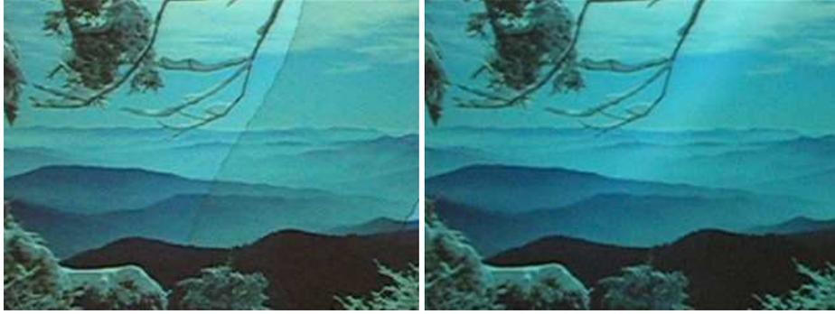
**Figure 18:** Boundary between regions of varying projector ownership. *Left:* before seam blending. *Right:* after seam blending.
