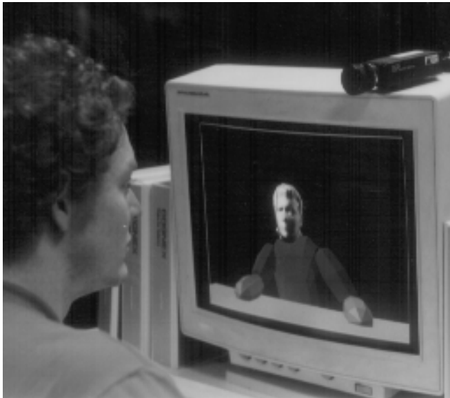
Fig. 2. The head tracking system in virtual holography mode, note camera at top of monitor.
