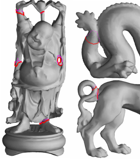
Fig. 9. This figure displays the non-separating cycles that are used for genus reduction for the Buddha (a), the dragon (upper-right), and the feline (lower-right). Each separating cycle consists of a sequence of edges in the surface that form a closed loop. Notice they appear in intuitive places. Furthermore, they tend to be short, smooth, and non-winding.
