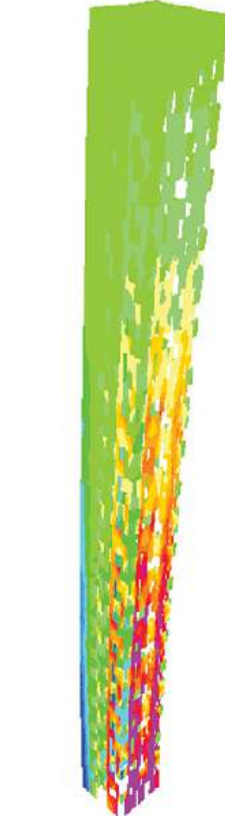
Stress plot of wind load in Y direction
